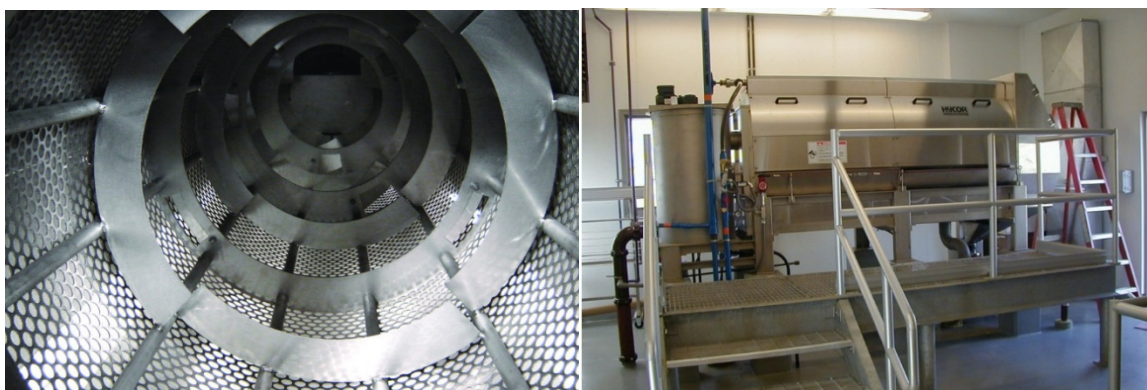
Figure 6: Example of Rotary Drum Thickener (Parkson Corporation)
