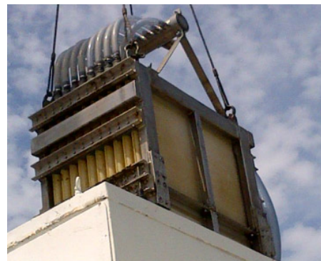
Figure 1: Membrane Bioreactor Example - Fibrecast FibrePlate (Fibrecast)
