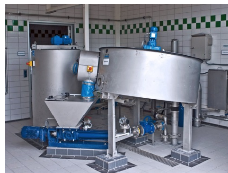
Figure 4: Disk Thickener (Huber, Inc.)
