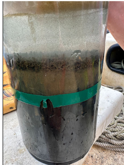
Figure 4.2 Sediment core collected under the southern aquaculture area on August. 29, 2023 showing the abundant amphipod tube mat covering the oxidized sediment surface.
