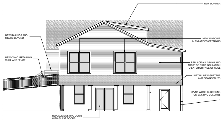
① SOUTH ELEVATION - PROPOSED 3/16" = 1'-0"
