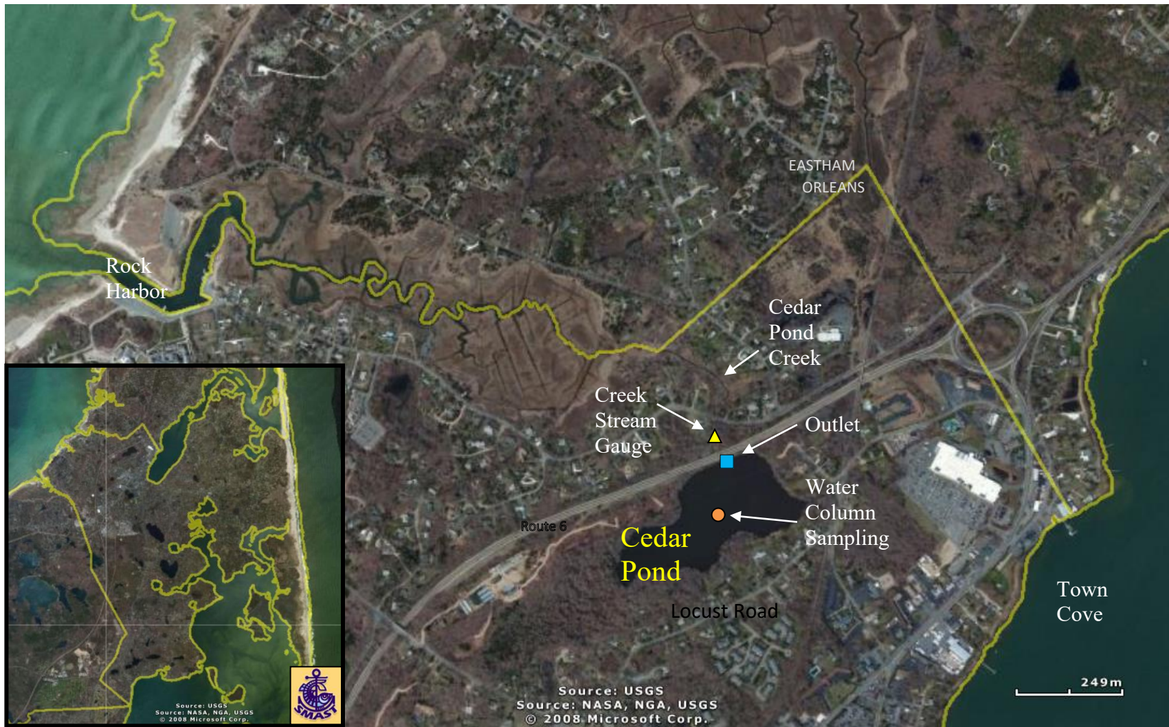
Figure I-1. Cedar Pond Locus in the Town of Orleans, MA. Cedar Pond is located in northern Orleans, south of Route 6 and west of Town Cove. The Pond is connected to the Rock Harbor estuary on Cape Cod Bay via Cedar Pond Creek. The creek leaves the pond through a weir at the pond outlet (blue square), flows under Route 6 and Rock Harbor Road, and through a salt marsh to Rock Harbor. Creek flow and water quality have been measured several times at the same location (yellow triangle) and the pond has been sampled regularly since 2000 at the same deep location (orange circle).
