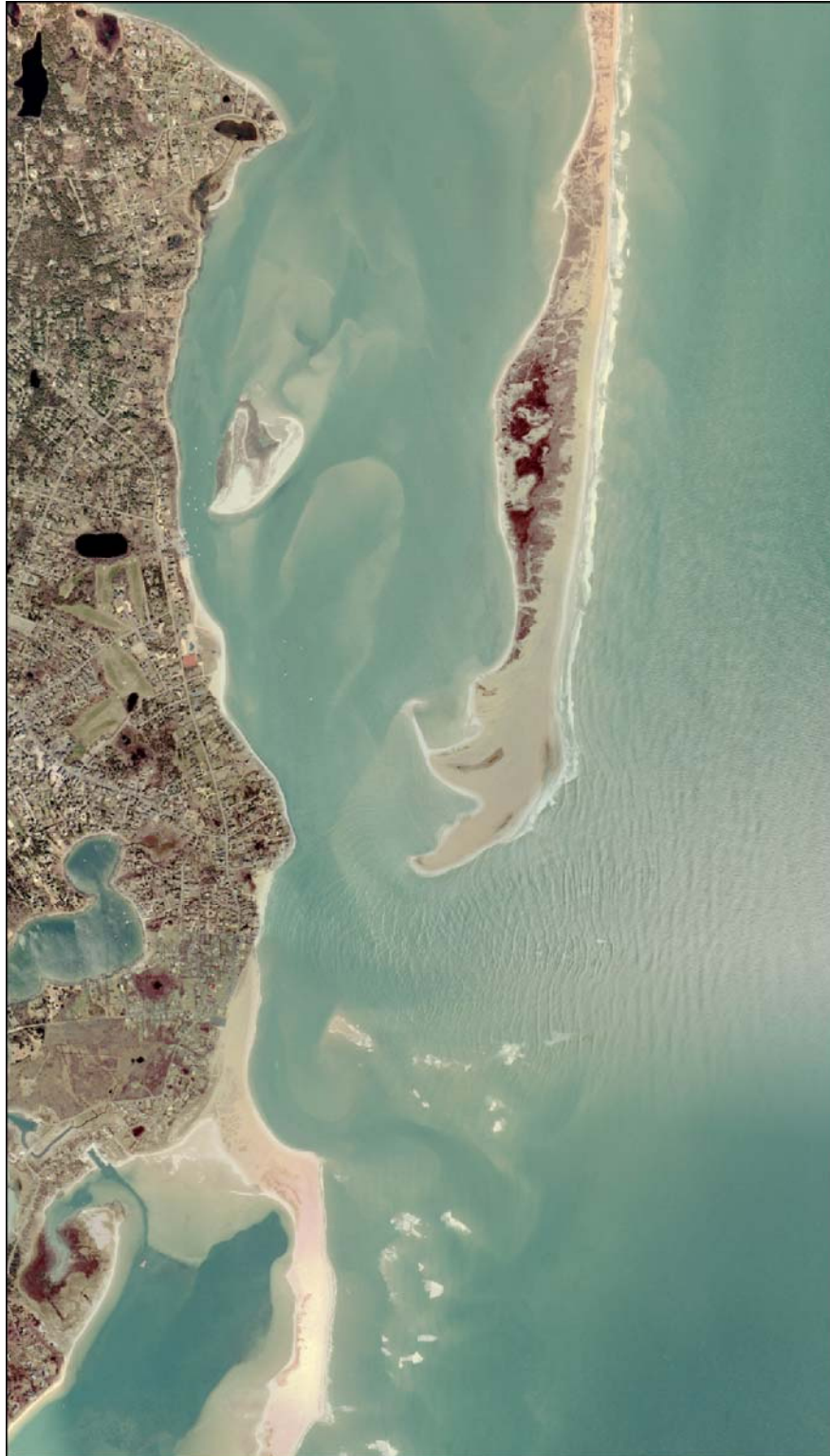
Figure V-6. Aerial photograph from April 2001 illustrating changes in the inlet geomorphology (source: MassGIS).
