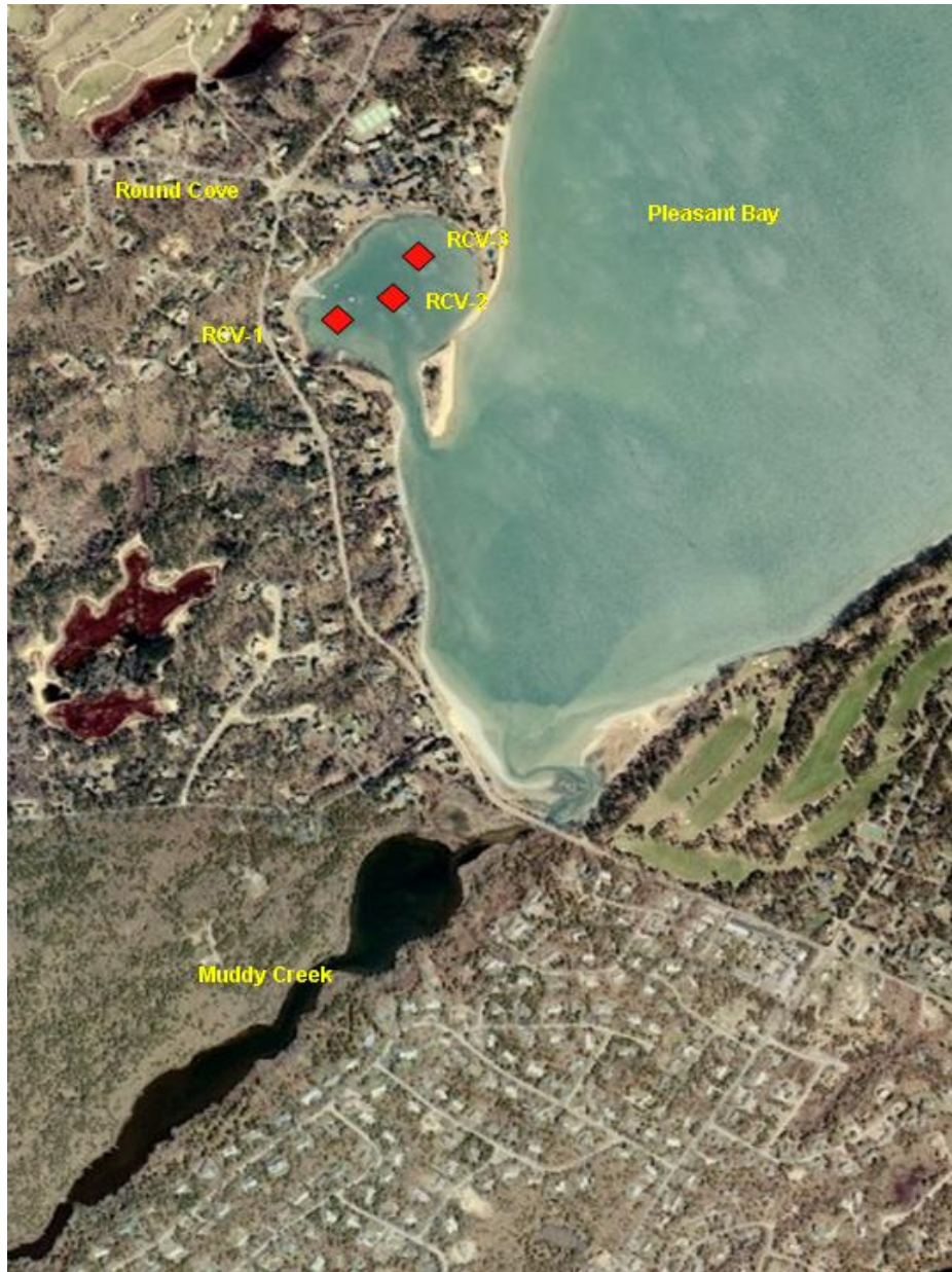
Figure VII-51. Aerial photograph of the Round Cove sub-embayment (Town of Harwich) showing location of benthic infaunal sampling stations (red symbols).
