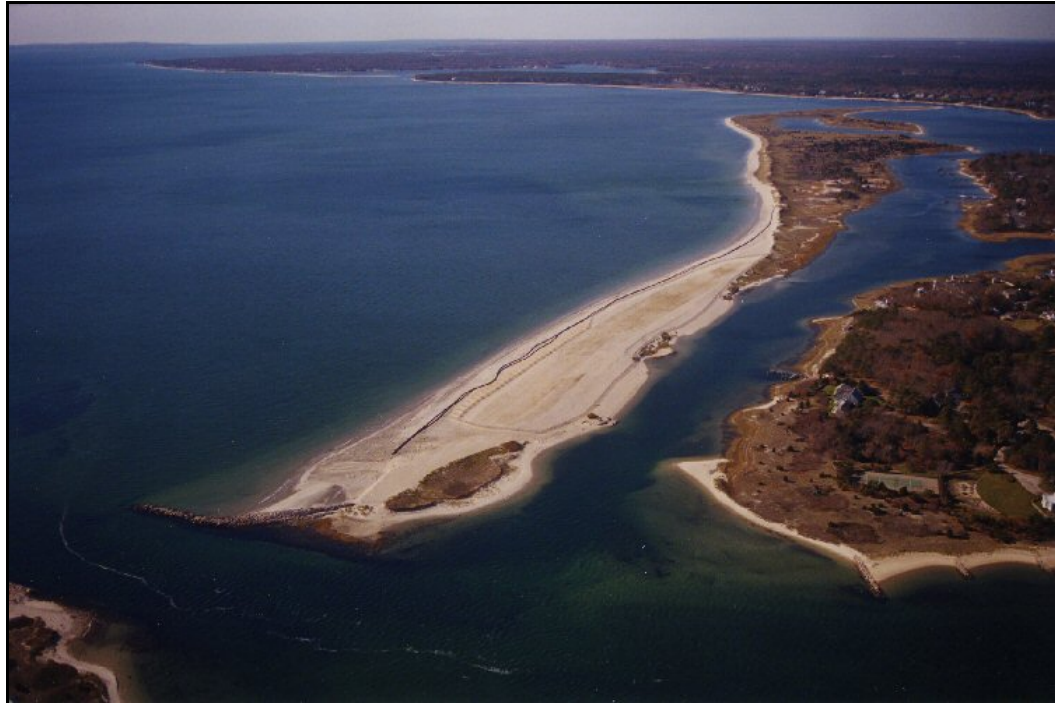
Figure V-6. Dead Neck Beach immediately following the beach nourishment in 2000, where the beach width had been increased significantly to prevent breaching of the barrier.
