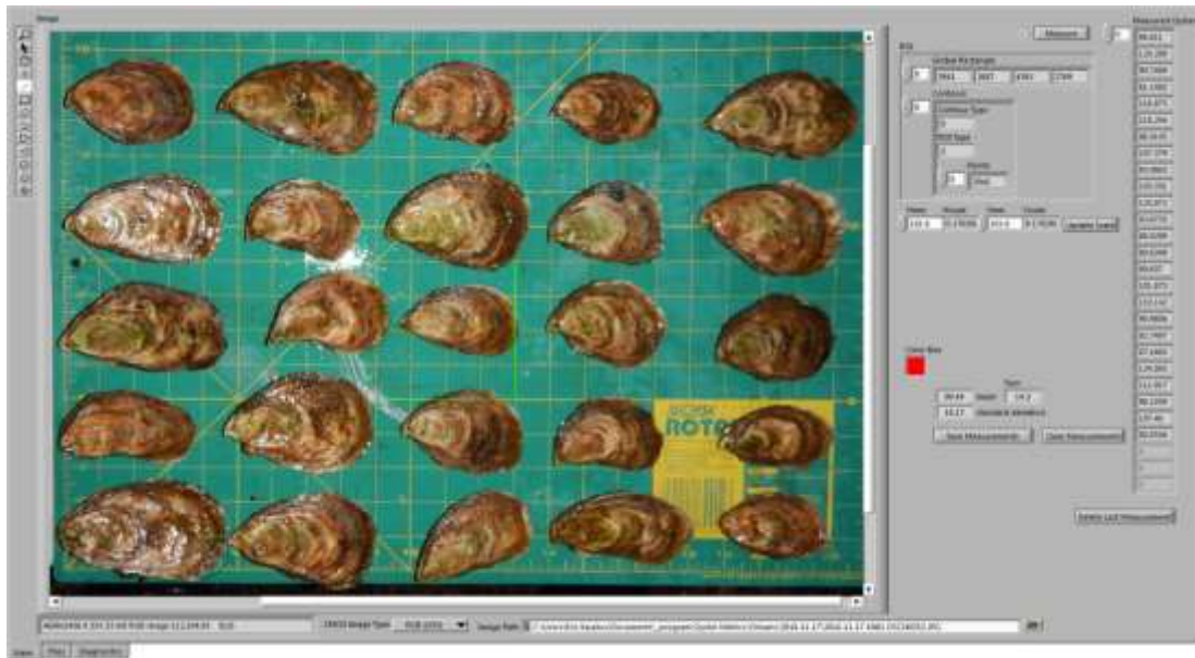
Figure 7 - Custom LabView Program for Measuring Oyster Length
