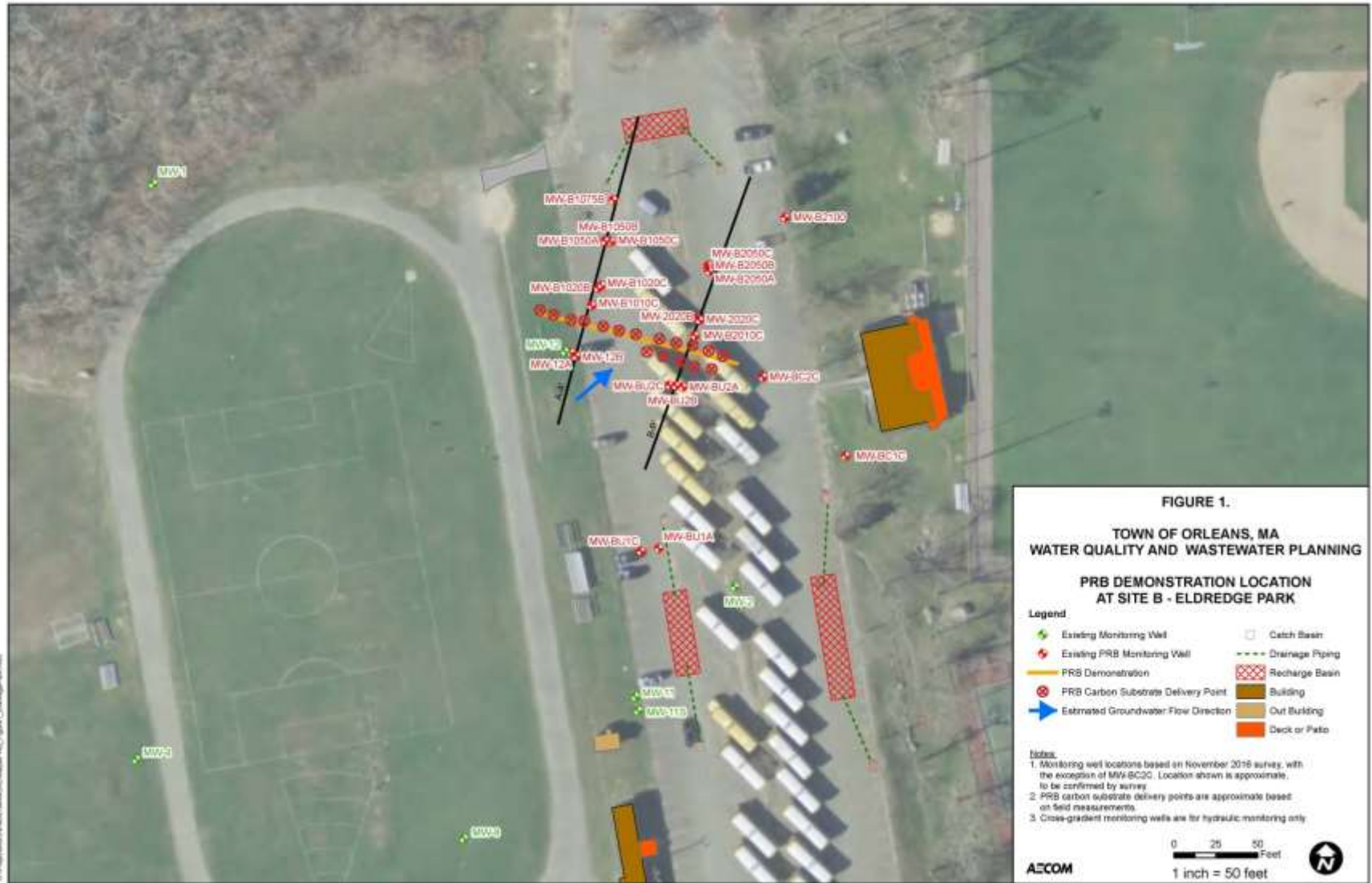
Figure 5-2 – Proposed PRB demonstration project at Eldredge Park showing locations of Monitoring Wells
