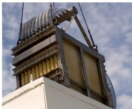
Figure 1: Membrane Bioreactor Example - Fibracast FibrePlate (Fibracast)
