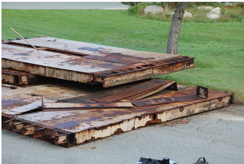
Failed Receiving Area Floor Scale Panels
