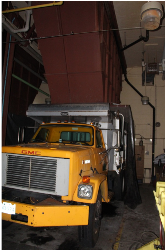
10-Wheel Dump Truck for Dewater Solids ("Cake") Transport
