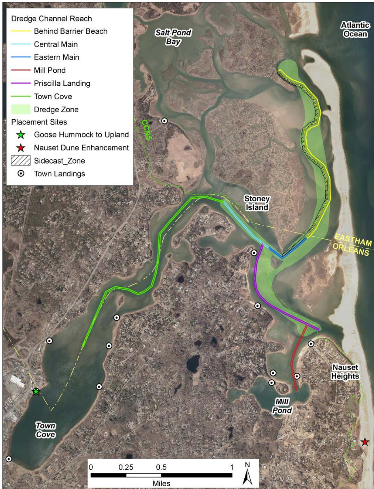
Figure B-2. Nauset Estuary Dredging project showing the preferred alternatives for channel layout, channel width and dredged material placement sites.
