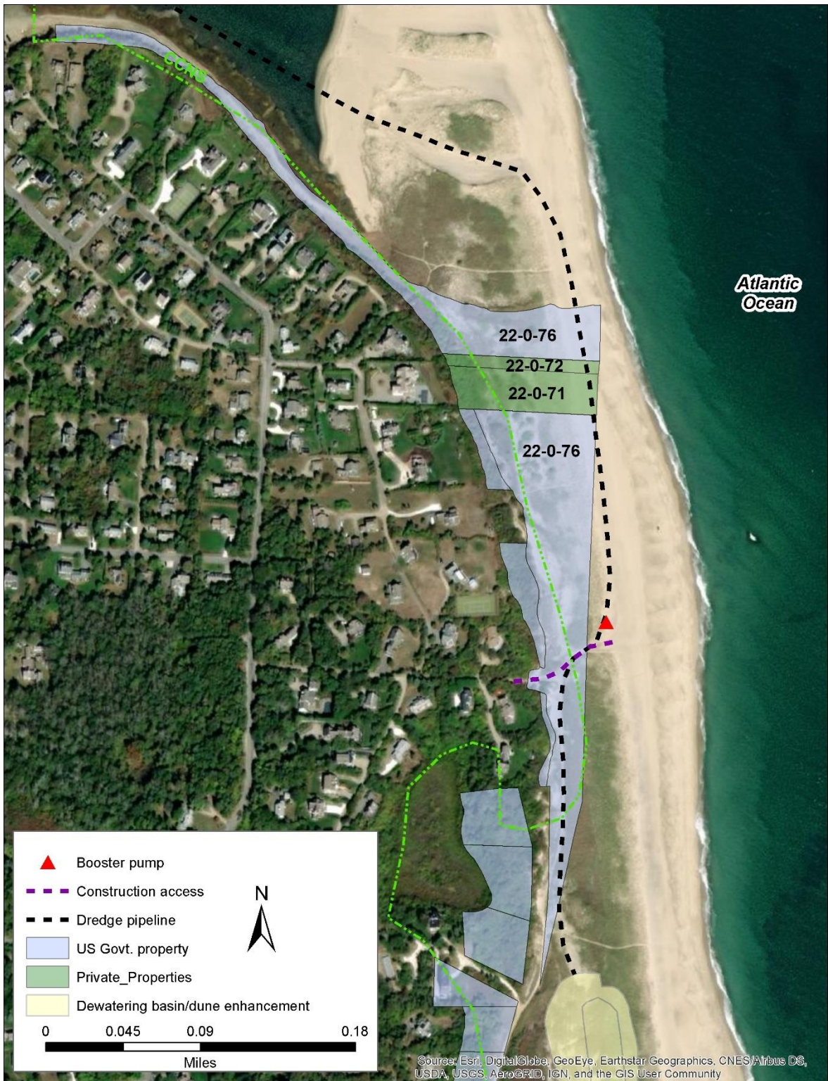
Figure 3. Dredge pipeline route between the Priscilla channel and the dewatering basin north of Nauset Public Beach. The dredge pipeline crosses property owned by the Town of Orleans (unshaded), US Government (shaded blue), and two private property owners (shaded green).
