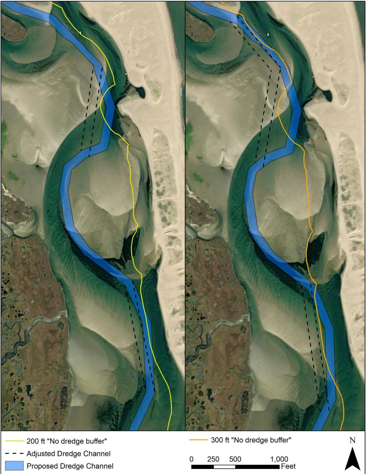
Figure 2. Adjustments to dredge channel required with 200-ft and 300-ft “no dredge buffers” off the back of the barrier beach.
