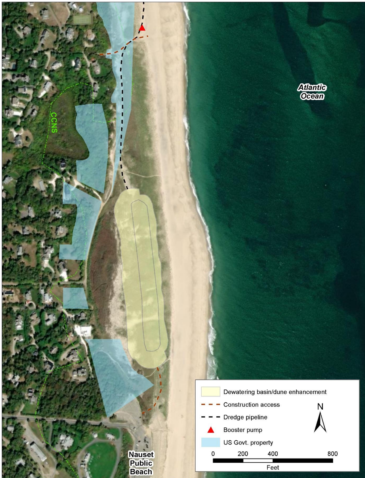
Figure 4. Proposed dewatering basin and dune enhancement area north of Nauset Public Beach.
