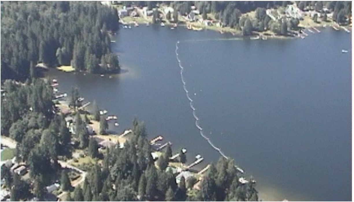
Photo 1: View of installed siltation barrier from above.
