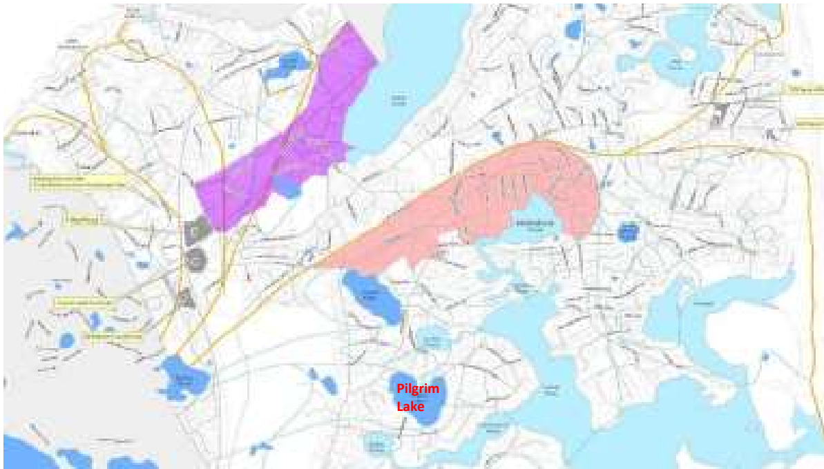
Figure V-1. 2016 Amended Draft CWMP Orleans Sewer Areas. Draft Amended Orleans Comprehensive Wastewater Management Plan (CWMP) shows sewerage planned for downtown area (purple) and within a portion of the Meetinghouse Pond watershed (pink). This draft plan does not show any planned sewerage properties within the watershed to Pilgrim Lake; sewerage would eliminate wastewater phosphorus additions to Pilgrim Lake and lower nitrogen loading to Lonnie's Pond (via herring run). Modified from draft Figure 5-1 in AECOM Technical Services, Inc. (2016).
