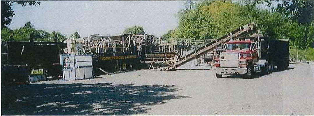
REPRESENTATIVE SMALL SCALE FILTER PRESS DEWATERING PLANT
