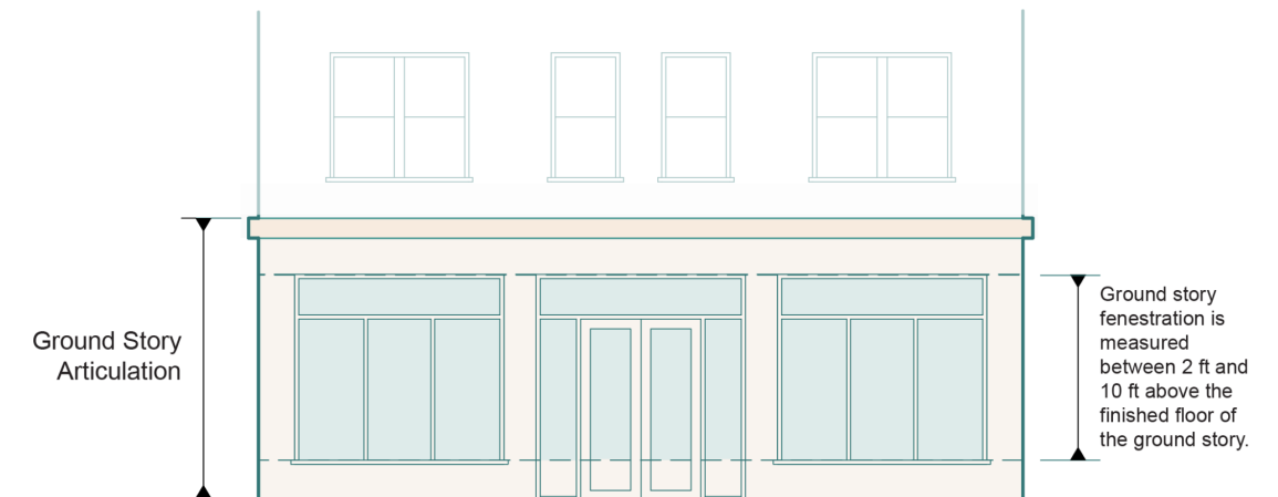
Figure 9. Ground Story Fenestration
