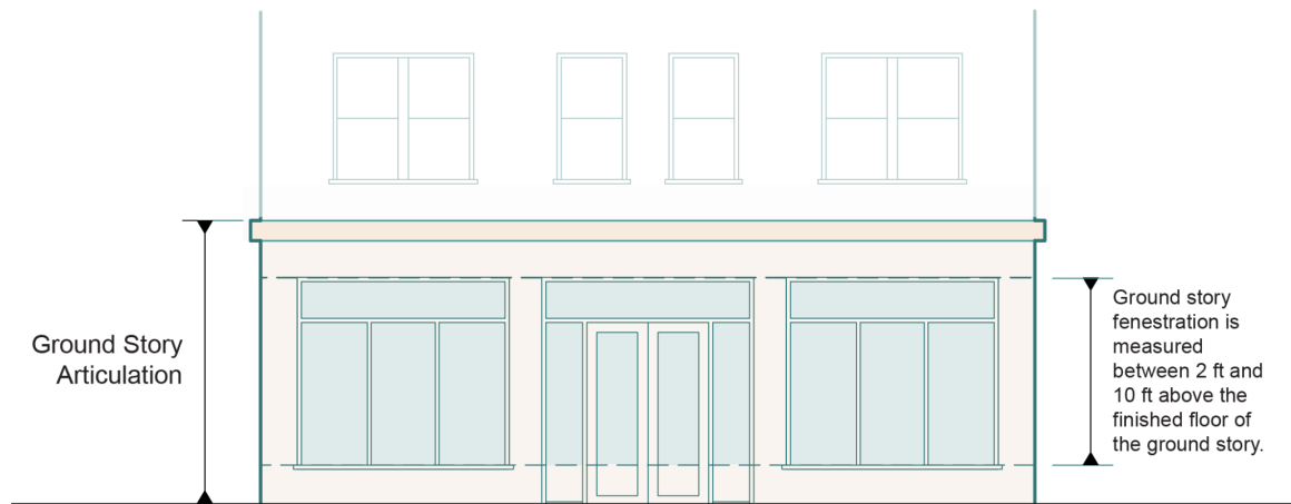
Figure 9. Ground Story Fenestration
